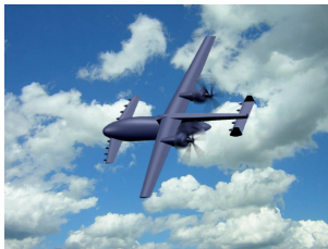
Fig. 1. Computer-aided design of UAV with vortex-active lifting surfaces
